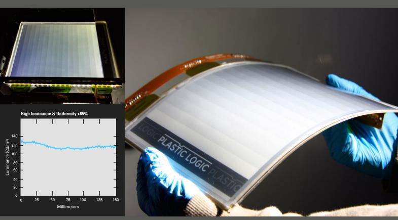
10.7" FLG laminated on a flexible e-paper display. In cooperation with Plastic Logic.
